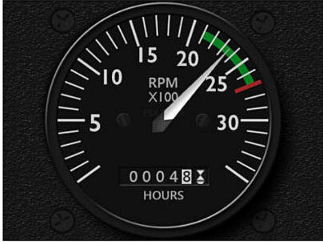
The image shows a circular RPM gauge for a Cessna C172SP. The gauge has a black face with white markings and numbers. The scale ranges from 0 to 30, with major markings every 5 units and minor markings every 1 unit. The needle is pointing to approximately 22. The text 'RPM X100' is printed in the center. Below the needle, there is a digital display showing '00048' and the word 'HOURS' below it. The gauge is mounted on a black panel with four screws.
